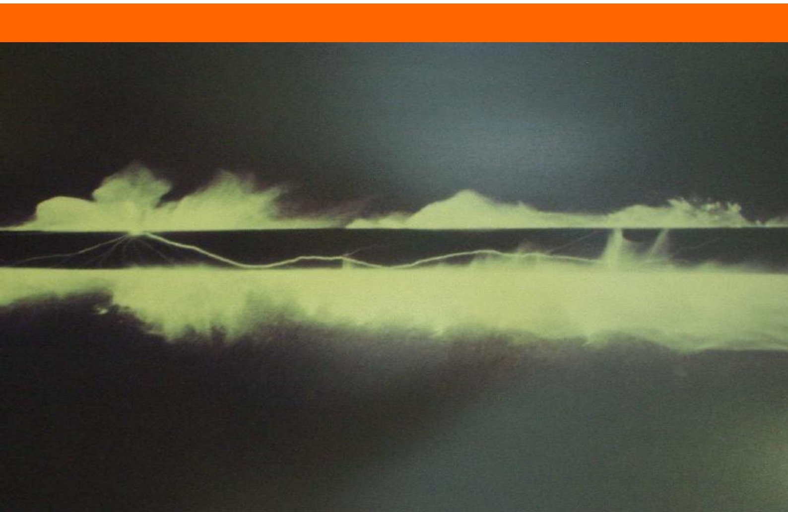
Figure: Propagating static discharge from a plastic pipe conveying diesel fuel
