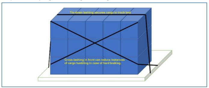
It must be ensured that the bed of trucks/trailer are in good condition & as flat as possible. Trucks with uneven bed will cause breakage to blocks during transit. In such case it is better to either throw soil on the bed or husk or cardboard sheets etc.
