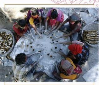
Until the mid-1980s, firecracker production was low-tech. They were handmade, beginning with rolling tubes. Once the firecracker tubes were rolled by hand (commonly from waste newspaper) and then filled with powder, their ends were crimped,
